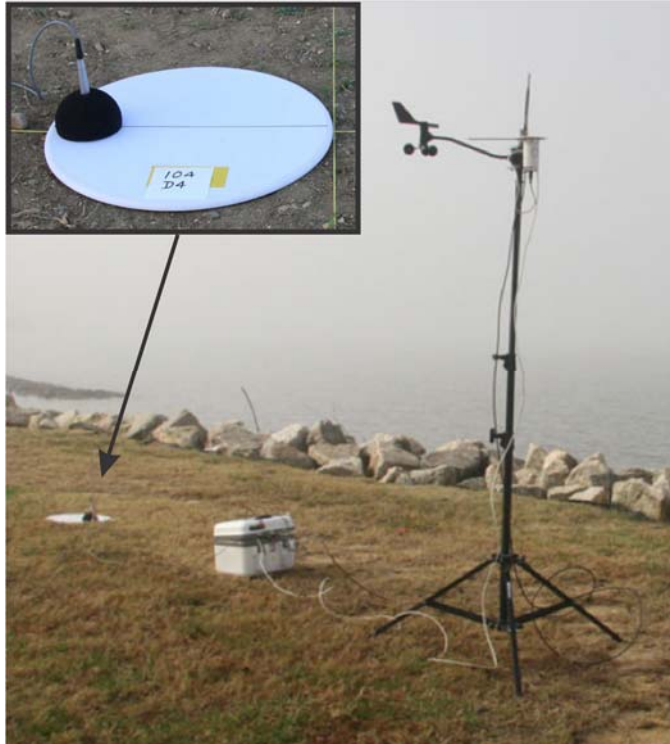
Figure 5. Typical WAMS microphone station deployment.
