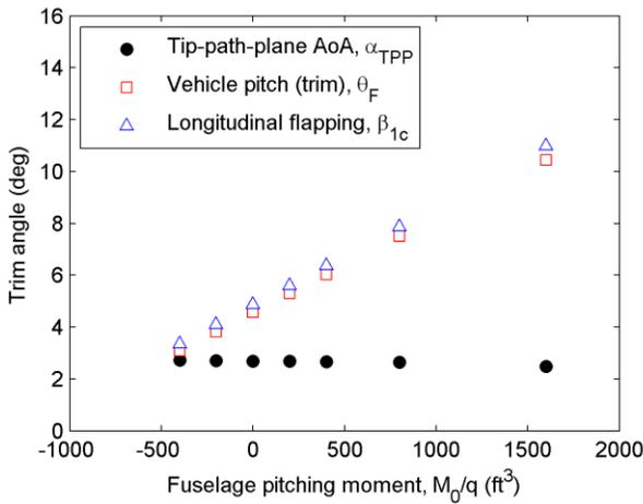
Figure 12. Effect of fuselage pitching moment on trim
