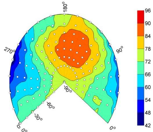
**Figure 5. BVI SPL at 500 ft for  $f = 87.4$  ft<sup>2</sup>**
